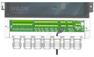
To stop the product dosing when there is no water circulation in the analysis chamber, the set has a flow detector connected to the control unit. This detector is connected to terminal block DI1, terminals 19 (+) and 21 (-) and terminal 20 (Signal).
