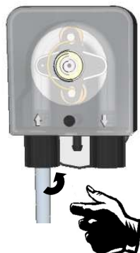
STEP 15 Unscrew the cap and pass the clear pipe
