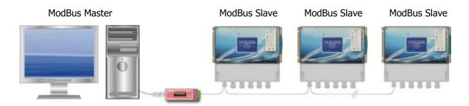
Connection of one or more TERE'O Touch controllers via the RS485 BUS...
