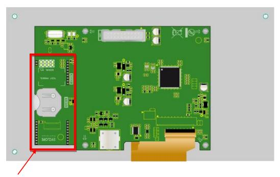
Socket Modem location for GSM, Wifi or Ethernet communication.
