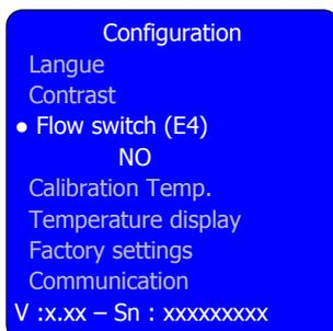
By pushing on **OK** key whereas the line **"Flow switch"** is in intensified brightness allows to have access to select the polarity of the circulation flow switch.
