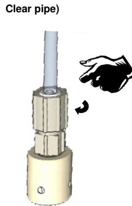
STEP 16 Tighten the nut on the cone...
