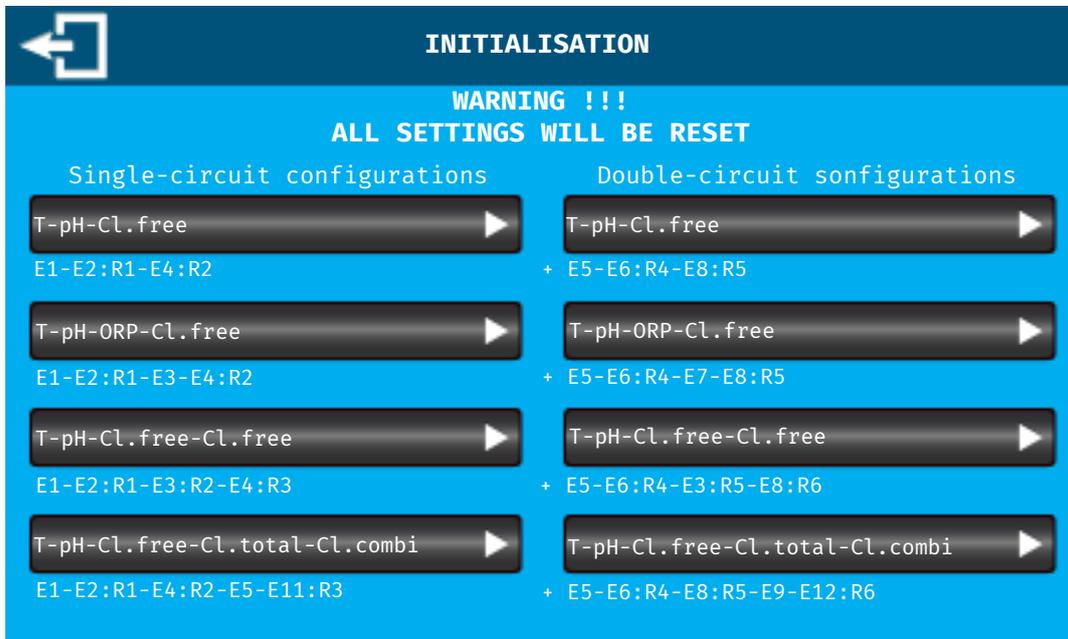
This screen allows you to make a "quick configuration" of your **SYCLOPE ALTICE'O®** controller. It is possible to choose from 8 different programs 4 single circuit and 4 double circuit
