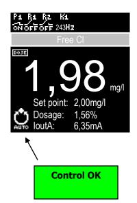
When polarization time done, the dosing control is activated.
