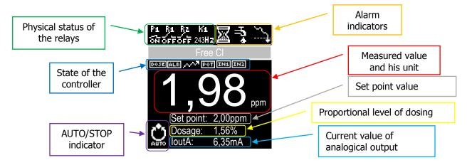
This screen allows you to display the good working of the process and to know:
