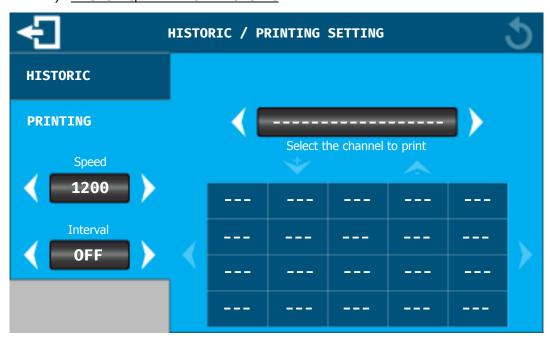
Printing allows the measurement values to be printed on the RS232 port at regular intervals.
