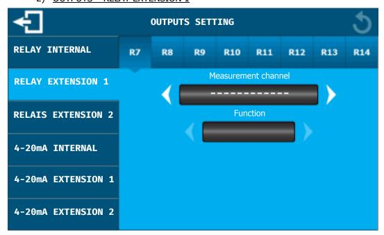
Refer to the previous section (RELAY INTERNAL) for the relay settings for extension module No. 1.
