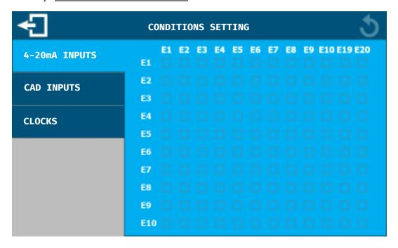
Depending on the configuration of the **SYCLOPE ALTICE'O**® controller inputs, some check boxes are enabled.
