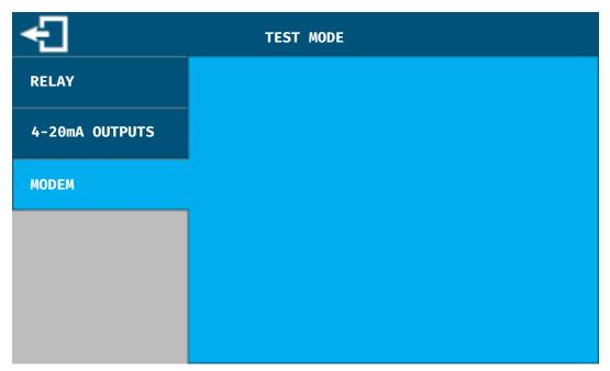
This screen allows you to view the status of the modem and validate the network connection.
