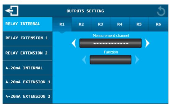
The upper band is used to select the relay output to be programmed.
