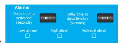
**Low alarm, high alarm, technical alarm:** By checking these boxes you can select the type of alarm that will be taken into account for relay switching.
