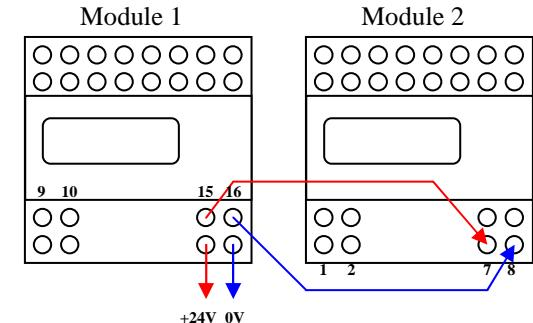
Maximal number of modules chained with « MODUPAC Power » module is finding out by maximal consummation of each acquisition module.
