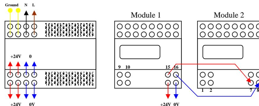
Maximal number of modules chained with « MODUPAC Power » module is finding out by maximal consumption of each acquisition module.
