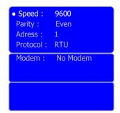
By using  $\uparrow$  and  $\checkmark$  keys allow to select the parameter to be modified, when the desired parameter is in intensified brightness. Press on **OK** key to enter in modification mode.
